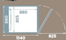
Carrier size: 880 x 805mm External dim: 1140 x 880mm Rated load: 250 kg / 2 persons
