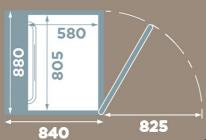
Carrier size: 580 x 805 mm External dim: 840 x 880mm Rated load: 250 kg/2 persons
